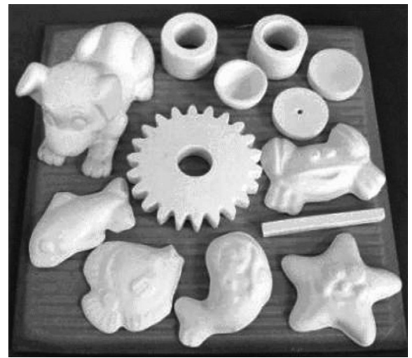
Fig. 9. Alumina dense ceramics obtained by pre-gelling starch consolidation.
